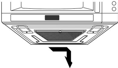
3. **Soak** grease filter in hot water and a mild detergent. **Scrub and swish** to remove embedded dirt and grease. **Rinse well and shake** to dry. **Do not clean filter with ammonia, corrosive cleaning agents such as lye-based oven cleaners, or place them in a dishwasher. The filter will turn black or could be damaged.**
