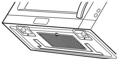
2. **Remove** the bulb cover mounting screws.
