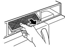
5. **Slide** a new charcoal filter into place. The filter should rest at the angle shown.
