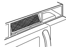
6. **Slide** the bottom of the vent grille into place. **Push** the top until it snaps into place. **Replace** the mounting screws.
