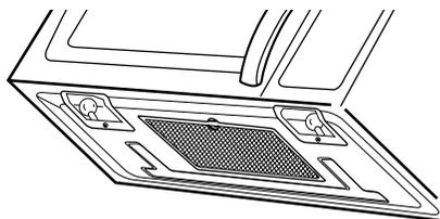
2. **Remove** the bulb cover mounting screws.
