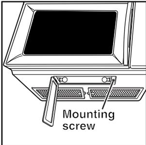
3. Remove the burnt-out bulb(s) and replace with 10W low-voltage halogen capsule bulb(s) (PN 8169418).\* Use a soft tissue to handle bulb(s), or wear a cotton glove. Do not touch bulb(s) with your bare fingers.
