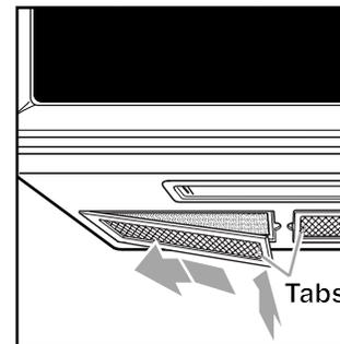
into the outer side of the filter opening. Make sure you are sliding in the side of the filter that does not have the tab. Hold the tab with your other hand. Push up the tab side of the filter and slide the filter to the other side of the opening to lock into place.
