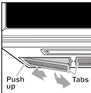
push each filter up on the side opposite the tab. Grasp the tab and slide the filter to the side. Pull the filter downward. It will drop out.
