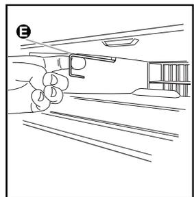
5. Grasp the microwave oven. Rotate the microwave oven downward. (Be careful that door does not swing open.)
