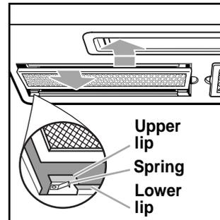
to the back of the opening, between the upper and lower lips against the springs. Swing the front of the filter up against the upper lip. Slide the filter forward while pushing it up against the upper lip. The filter will now be held in position between the lips by the spring.
