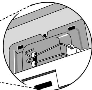
5. Remove the burnt-out bulb by squeezing the wire clip together, pulling to the right and lifting up. Replace the bulb with a 10W low-voltage halogen capsule bulb (PN 8169418).\* Use a soft tissue to handle the lamp, or wear a cotton glove. Do not touch lamp with your bare fingers.
