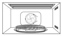
We recommend preheating the oven before placing food inside for cooking. When the microwave oven is preheated, place cookware containing food on the convection grid or place food directly on the grid. Prevent heat loss by opening the door only when necessary and closing it quickly during CONVECT cooking.
