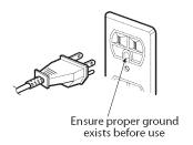
▲ WARNING: Improper grounding can result in a risk of electric shock. Consult a qualified electrician or service technician if you do not understand the grounding instructions, or if you wonder whether the appliance is properly grounded. Do not use an extension cord. If the power supply cord is too short, have a qualified electrician or service technician install an outlet near the microwave oven.
