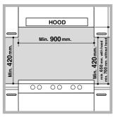
• If the cooker is installed underneath a wall cabinet, there must be a minimum distance of 420 mm between this cabinet and the top of the hob.
