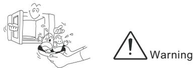
Remember to clear away excess grease from the inside the cavity. Otherwise it may cause smoke or fire during heating.
