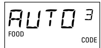
Beep sounds when steam is sensed and “AUTO” is replaced by cook time. Rotate or stir food, if necessary. When done, oven beeps every minute until door is opened or CLEAR/OFF is touched.
