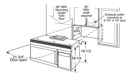
Note: Requires 120V grounded outlet. Electrical receptacle must be located in cabinet above SpacemakerXL microwave oven. No additional wiring, venting or cabinet rebuilding necessary in many cases. Complete detailed, easy-to-follow installation instructions and convenient full-size templates are packed with the SpacemakerXL microwave oven.
