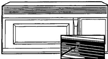
To replace your oven light, first **disconnect power at main fuse or circuit breaker panel or pull plug.** Remove the top grill by taking out the 2 screws that hold it in place.
