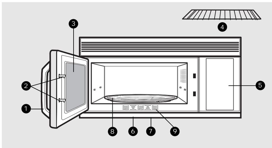
**1 Door Handle.** Pull to open the door. The door must be securely latched for the microwave to operate.
