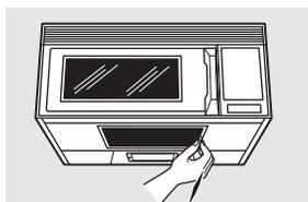
**To remove**, slide it to the rear using the tab. Pull it down and out.
