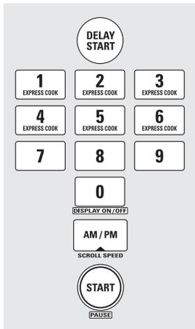
Delay Start allows you to set the microwave to delay cooking up to 24 hours.
