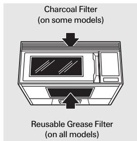
The vent fan has 1 metal reusable grease filter.
