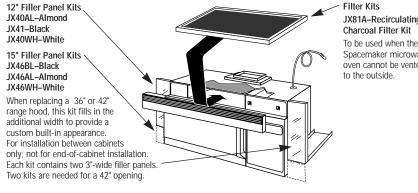
JX81A-Recirculating To be used when the Spacemaker microwave oven cannot be vented
