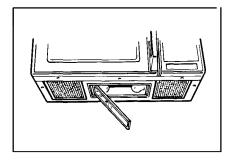
Be sure bulbs to be replaced are cool before removing. Break the adhesive seal by gently unscrewing the bulbs. Replace with 40-watt incandescent bulbs (Part No. WB2X4253) available from your GE supplier. High intensity 40-watt bulbs (Part No. 40S11N/1) which are available in supermarkets and hardware stores may also be used for replacements. Raise light compartment cover and replace screw. Connect electrical power to microwave oven.
