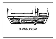
To replace cooktop light in hood, first disconnect power at main fuse or circuit breaker panel or pull plug. Remove screw on right side of light compartment cover and lower cover until it stops.
