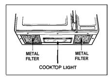
The exhaust hood feature on your microwave oven is equipped with two metal filters which collect grease. When the fan is operated, air is drawn up through the filters and is then discharged through the provided venting to the outside. The hood also has a light for illuminating the counter space.
