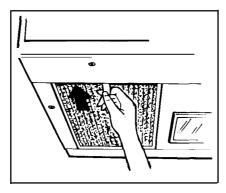
Pull filter upward and to the front to lock into place.
