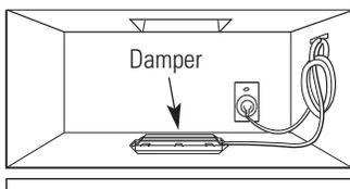
**4** Use the power supply cord clamp to bundle the power supply cord. Install the power supply cord clamp, using a screw as shown, to the inside of the cabinet.
