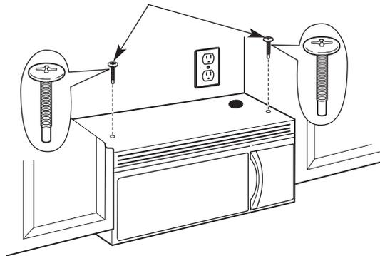
**7** Tighten the two screws to the top of the microwave oven. (While tightening screws, hold the microwave oven in place against the wall and the top cabinet.)
