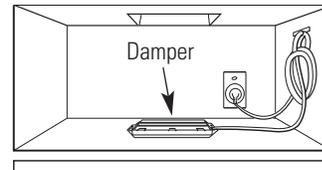
**4** Use the power supply cord clamp to bundle the power supply cord. Install the power supply cord clamp, using a screw as shown, to the inside of the cabinet.
