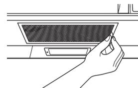
**8** Install grease filter. See the Owner's Manual packed with the microwave oven.
