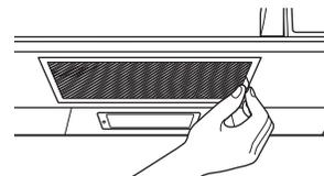
**8** Install grease filter. See the Owner's Manual packed with the microwave oven.
