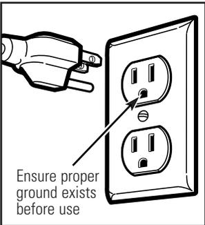
The power cord of this appliance is equipped with a three-prong (grounding) plug which mates with a standard three-prong (grounding) wall receptacle to minimize the possibility of electric shock hazard from this appliance.
