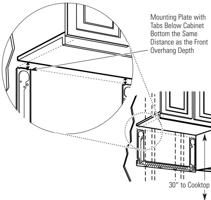
Your cabinets may have decorative trim that interferes with the microwave oven installation. Remove the decorative trim to install the microwave oven properly and to make it level.
