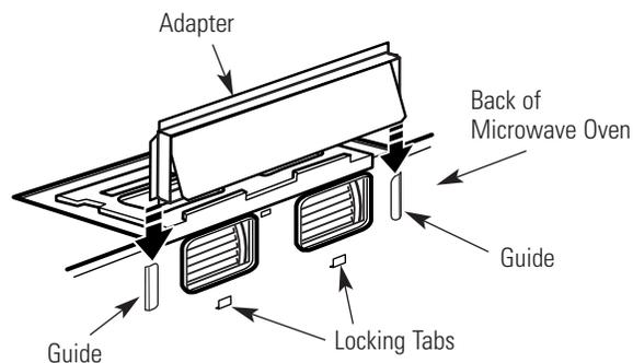
Push in securely until it is in the lower locking tabs. Take care to ensure that the damper hinge is installed so that it is at the top and that the damper swings freely.
