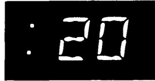
After the popcorn sensor detects steam, the oven signals and displays remaining cooking time needed.
