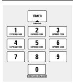
Timer On/Off operates as a minute timer and can be used at any time, even when the oven is operating.
