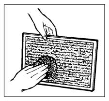
To clean grease filter, soak, then agitate filter in hot detergent solution. Don't use ammonia or other alkali because it will darken metal. Light brushing can be used to remove embedded dirt. Rinse, shake and remove moisture before replacing. Filters should be cleaned at least once a month. Never operate your hood without the filters in place. In situations where flaming might occur on surfaces below hood, filters will retard entry of flames into the unit.
