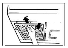
Then pull filter downward and to the front. The filter will drop out
