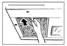
Pull filter upward and to the front to lock into place.
