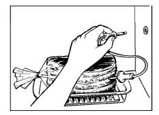
Place meat in oven with probe to the right. Insert cable end of probe firmly into receptacle on oven wall.
