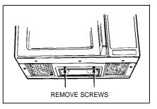
To replace cooktop light, first disconnect power at main fuse or circuit breaker panel or pull plug. Remove 2 screws in front of lamp cover. Lamp cover is hinged and will drop down. Be sure bulbs to be replaced are cool before removing. Remove bulbs and replace with 40-watt incandescent bulbs (WB2X4253) available from your GE supplier. Raise lamp cover and replace screws that were removed. Connect electrical power to microwave oven.
