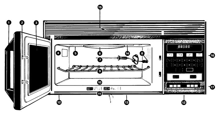
**1. Door Handle.** Pull to open door. Door must be securely latched for oven to operate.
