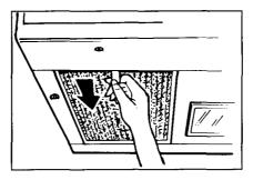
**To remove grease filter,** grasp the "finger hold" on the filter and slide to the rear.
