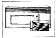
**To remove the charcoal filter, disconnect power at main fuse or circuit breaker or pull plug.** Remove the top grill by taking off 3 screws which hold it in place. Grasp filter and slide toward front of oven. It will slide right out.
