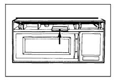
Next, remove the single screw located above door near center of oven that secures lamp housing. Remove bulb and replace with 30-watt incandescent bulb (WB2X4235) available from your GE supplier. Secure lamp housing with screw.
