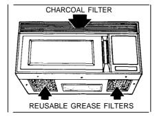
Your microwave oven has two reusable metal filters to help remove grease from the air and a disposable charcoal filter to help remove smoke and odors caused by cooking with your range. When the fan is operated, air is drawn up through the filters and then recirculated.
