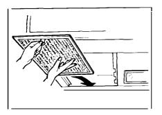
To replace grease filter, slide the filter in the frame slot on the back of the opening.
