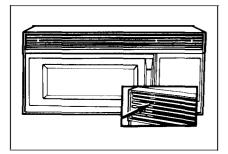
To replace your oven light, first disconnect power at main fuse or circuit breaker or pull plug. Remove the top grill by taking off 3 screws which hold it in place.
