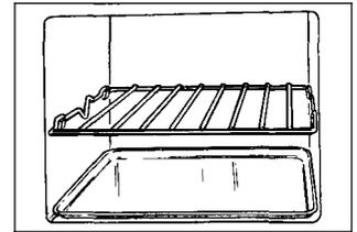
When properly positioned, the shelf should fit snugly in place, be level and not touch the back or side wall of the oven.
