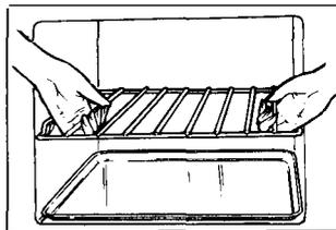
Next, lower the front until the shelf support guides fit **onto** the support guides located at each side of the oven in the front.
