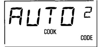
The beep sounds when the steam is sensed and "AUTO" is replaced by cook time. Rotate or stir the food, if necessary. When done, the oven beeps every minute until the door is opened or CLEAR/OFF is touched.
