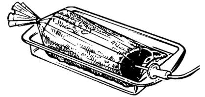
Place meat in oven with probe to the right. Insert cable end of probe firmly into receptacle on oven wall.
