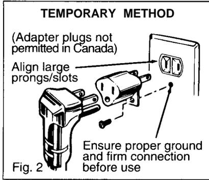
**Caution:** Attaching the adapter ground terminal to the wall receptacle cover screw does not ground the appliance unless the cover screw is metal, and not insulated, and the wall receptacle is grounded through the house wiring. You should have the circuit checked by a qualified electrician to make sure the receptacle is properly grounded.
