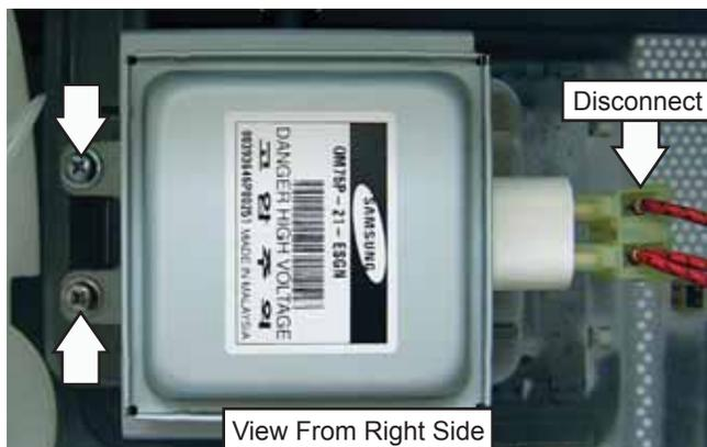
4. Disconnect wiring to the magnetron TCO.
