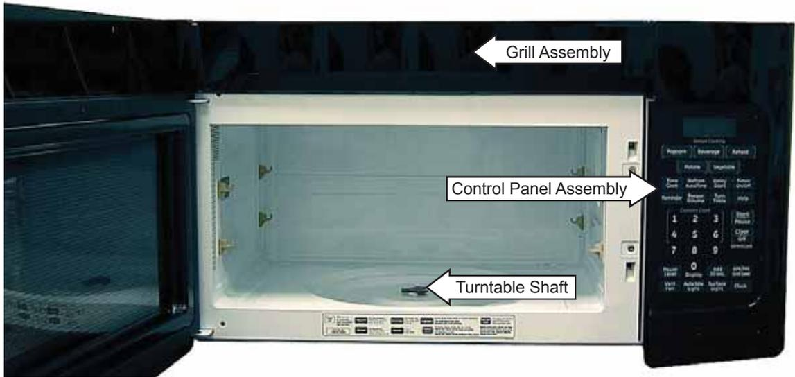
Front View - Control Panel Assembly Removed
