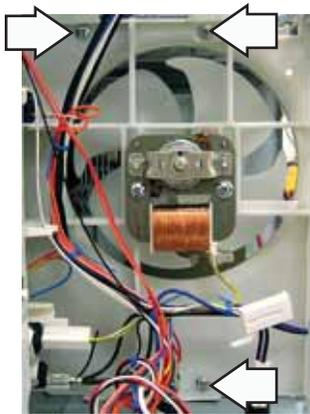
9. Remove 2 Phillips-head screws that attach the fan motor to the cooling fan frame.
