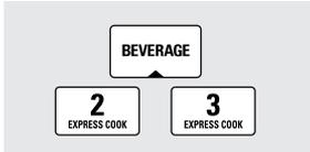
*On some models*, the serving size is automatically set at 1, but can be changed by pressing 2 or 3 right after pressing BEVERAGE.
