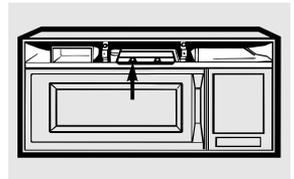
**4** Replace the screw. Connect electrical power to the oven.
