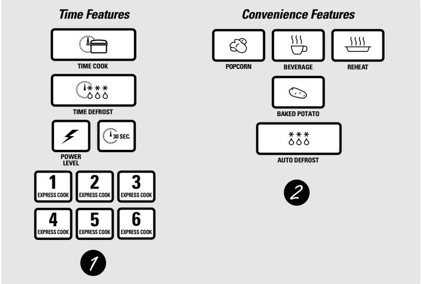
The diagram illustrates the control panel features of a microwave oven, divided into two main sections: Time Features and Convenience Features.
