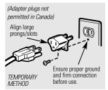
The larger slot in the adapter must be aligned with the larger slot in the wall receptacle to provide proper polarity in the connection of the power cord.
