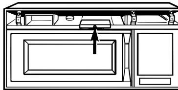
Next, remove the single screw located above door near center of oven that secures light housing. Replace burned-out bulb with a 40-watt incandescent bulb (WB02X4253), available from your GE supplier.
