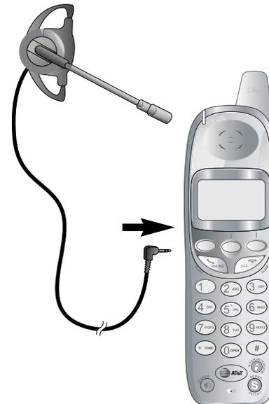
Plug 2.5 mm headset into jack on side of handset (beneath small rubber cap)
