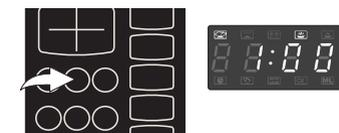
4. Press the **Power** button; the Microwave and High Cook indicators will light and “PL 10” will light in the display.
