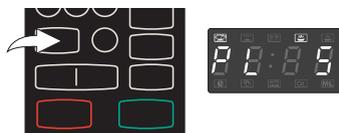
6. Press number keys to set the desired cooking time. (up to 99 minutes 99 seconds).
