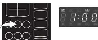
2. Repeatedly press the **+ 30SEC.** button to increase the cooking time in 30 seconds increments. (up to 99 minutes 59 seconds).
