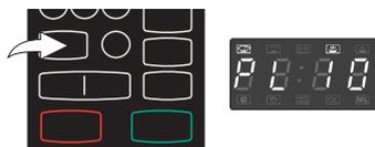
5. Press the **Power** button different times to set the desired power; the display will show the level of power you chose.
