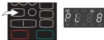
3. Press number keys to set the desired cooking time. (up to 99 minutes 99 seconds).
