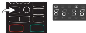
2. Press the **Power** button different times to set the desired power; the display will show the level of power you chose. If selecting power level 70%-10%, the Low Cook indicator will light instead of the High Cook indicator.
