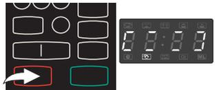
2. To deactivate, press and hold the **Stop/Cancel** button for three seconds, the display will return to the time.
