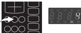
3. Follow one steps on the previous page (**COOKING IN ONE STAGE**) to set a second stage, then press the **Start** button to start cooking; the display will countdown the remaining time in minutes and seconds and beep once between stages. It will beep five times when all the stages have completed cooking.
