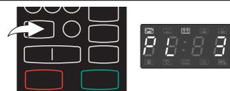
4. Press the **Start** button to start defrosting; the Microwave and Defrost indicators will blink and the display will show count down the remaining defrosting time in minutes and seconds. It will beep five times when defrosting is completed.
