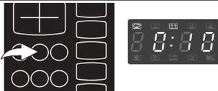
3. The default microwave power is power level 3. If you want to change the power level, press **Power** button once, and the LED will display "PL 3", then press the number keys of the power level wanted.
