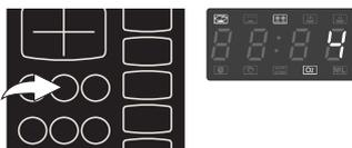
3. Press the **Start** button to start defrosting; the Microwave and Defrost indicators will blink and the display will countdown the remaining defrosting time in minutes and seconds. It will beep five times when defrosting is completed.
