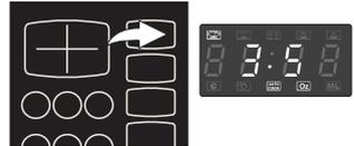
3. Press the **Start** button to start cooking; the Auto Cook indicator will blink and the display will countdown the remaining cooking time in minutes and seconds. It will beep five times when cooking is completed.
