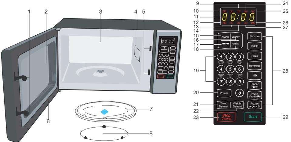
1. Door latch-When the door is closed, it will automatically lock shut. If the door is opened while the oven is operating, the magnetron will automatically shut off.
