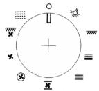
This commutator activates the desired cooking function. The illustration below shows the heat source and heat distribution for each selected operating mode. The lower and circular heating elements are housed in the bottom and rear end of the muffle respectively. The heating elements turn on/off automatically to maintain the desired cooking temperature.
