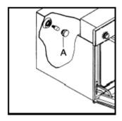
Prior to replacing the oven lamp, verify that the mains electricity has been disconnected by pressing the mains switch.
