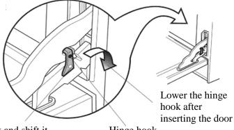
Lift the hinge hook and shift it into the locking indentation to remove the oven door
