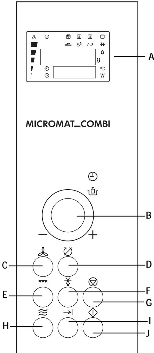
**A Display** for time of day, function, programme length, power level, temperature, weight, food type, etc.
