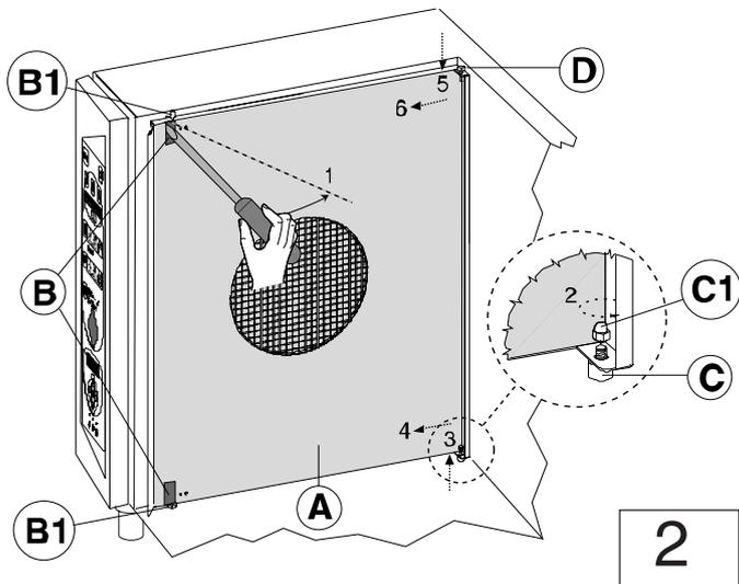
To refit the air intake wall, repeat the steps in reverse order and retighten nut C1.
