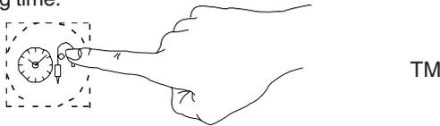
The relative DISPLAY will show the TOTAL REMAINING TIME of the cooking cycle (large numbers) and the TIME TO BE SET (small numbers - flash for 5 seconds).
