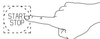
If this button is pressed for less than 2 seconds it will produce no result.
