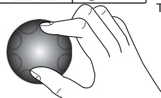
Turn the knob clockwise (to increase the value) or counter clockwise (to decrease the value) to set the desired COOKING TEMPERATURE in the small DISPLAY.
