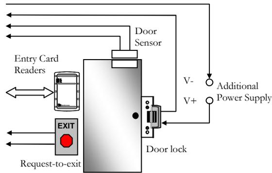
Fig. 1.2 A Common Door Configuration with Entry Reader
