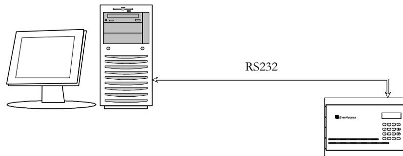
Figure 3.1 Connecting the Controller to a PC
