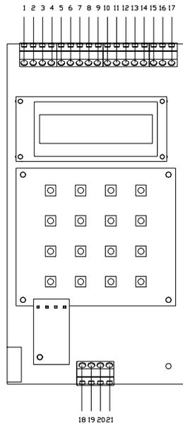
Figure 2.3 The main module and its terminals
