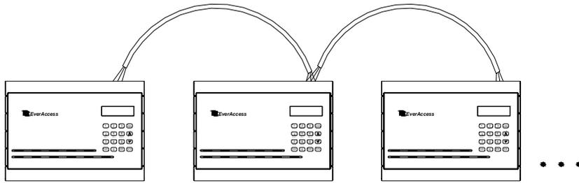
Figure 3.6 The Daisy Chain Connection Controller to Controller
