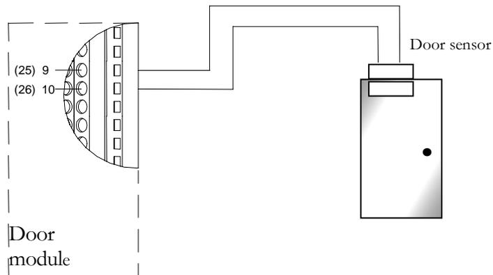
Fig. 2.12 Example for Connecting Door Sensor to Controller
