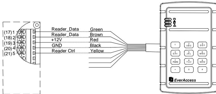
Figure 2.9(b) Connection to the EverAccess Reader using Wiegand Format
