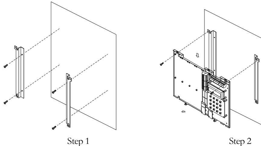
Step 2. Mount the controller base board.
