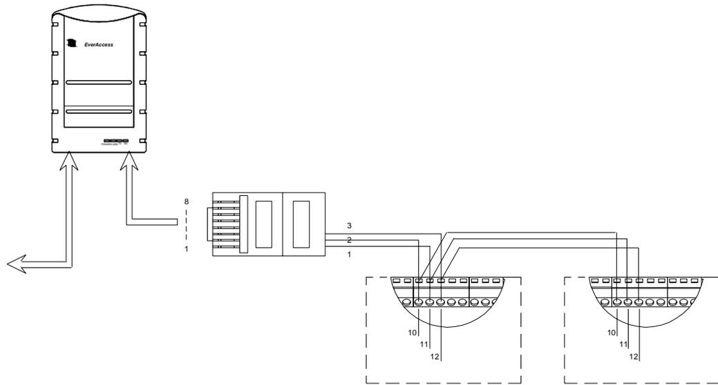
Fig. 3.8 Connection to Multiple Controllers via RS485
