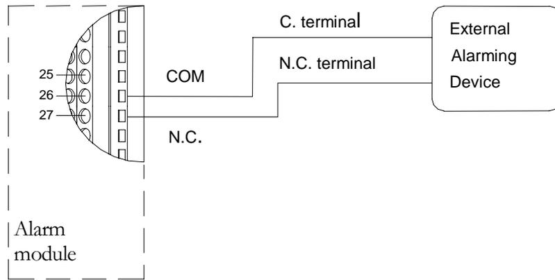
Fig. 2.16 Normally Closed Connections for Alarm Output 5
