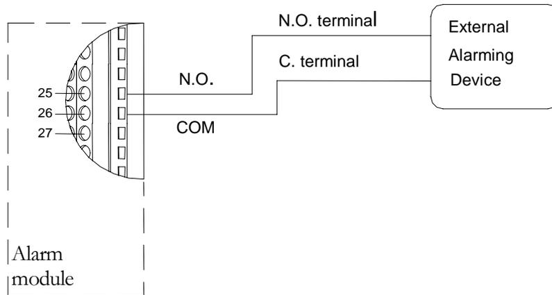
Fig. 2.15 Normally Open Connection for Alarm Output 5
