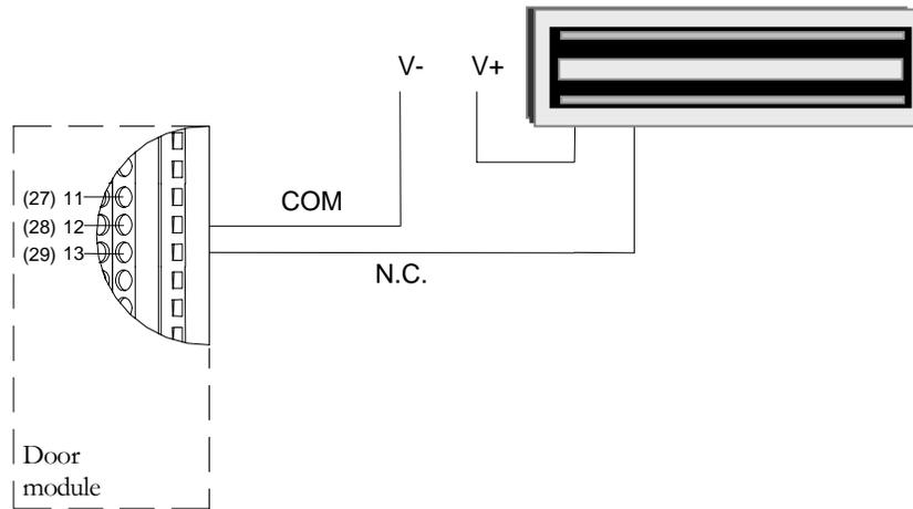
Fig. 2.11 Example for Connecting a Magnetic Lock
