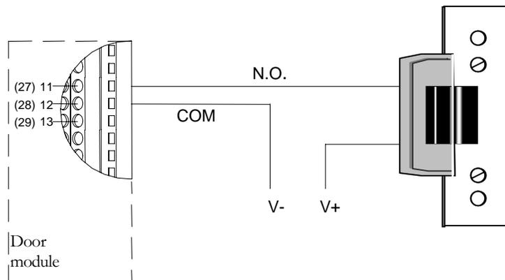
Fig.2.10 Example for Connecting an Electric Strike
