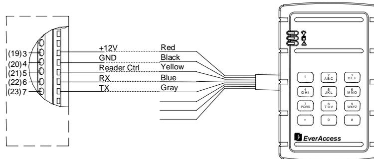
Fig. 2.9(a) Connection to the EverAccess Reader using RS232 Format
