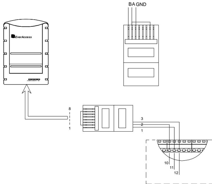
Fig. 3.3 Connection to Desktop Reader via RS485
