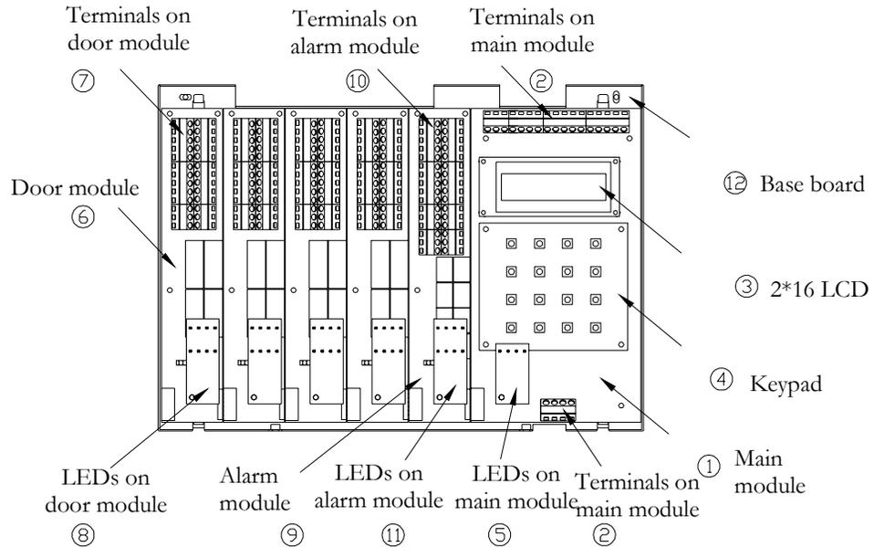
Fig. 1.1 Controller Layout
