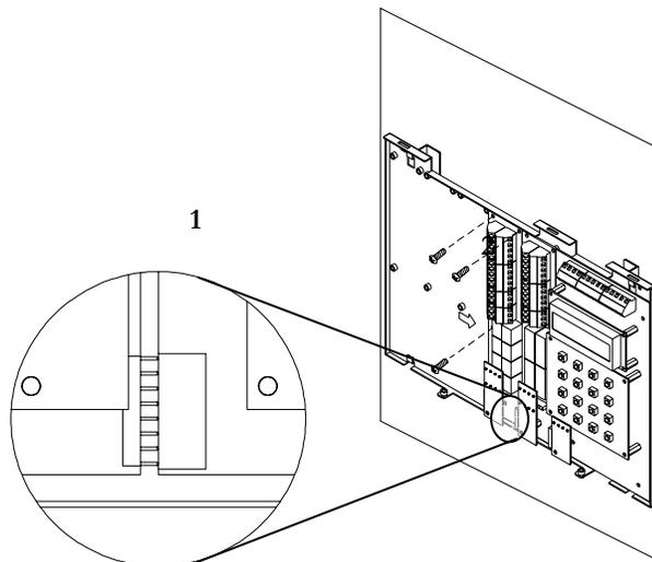
Figure 2.1 Install a New Module to Controller
