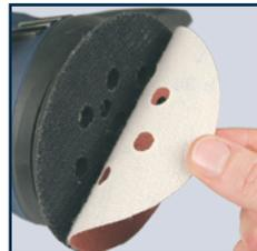
**CAUTION.** Take care to regularly clean out the build up of dust on the base underneath the sandpaper and not to let the sandpaper wear completely down before replacing it. Failure to observe these two precautionary measures can lead to damage to the hooks and loops on the platen and the sandpaper will not attach properly.
