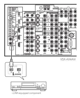
• The arrow on the cable connector body should be lined up with the arrow (to the left of the connector) on the receiver for correct alignment. The i.LINK cable should be inserted straight into the connector so that it snaps easily into place. If not connected properly the receiver will not be able to recognize any connected components. Note that the i.LINK cable is fragile and can be broken easily if too much force is used when connecting.
