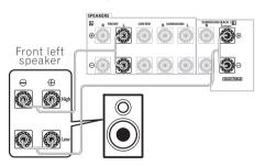
Since both front and surround back speaker terminals output the same audio, it doesn't matter which set (front or surround back) is powering which part (**High** or **Low**) of the speaker.
