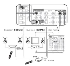
Different sources can be playing in three rooms at the same time or, depending on your needs, the same source can also be used. The main and sub rooms have independent power (the main room power can be off while one (or both) of the sub rooms is on) and the sub rooms can be controlled by the remote or front panel controls. However, you may need to specify the volume settings in *Multi-Room and IR receiver setup* on page 62.
