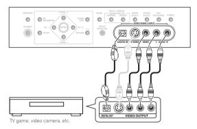
Select these inputs using INPUT SELECT (remote) or the INPUT SELECTOR dial (front panel) to select VIDEO/GAME 2.
