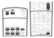
**1 Switch on your system components and receiver.** Start by switching on the playback component (for example a DVD player), your TV<sup>1</sup> and subwoofer (if you have one), then the receiver (press **& RECEIVER**).
