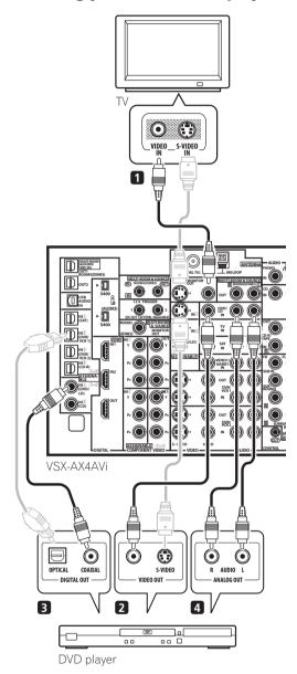
The diagram shows a basic setup of this receiver together with a TV and DVD player, with S-video or composite video connections. Different TVs and DVD players may offer alternative connections. See also *Using the*
