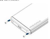
**2** Remove the plastic end cap and circuit board.
