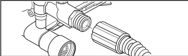
3. Run water through your garden hose for 30 seconds to clean out any debris.
