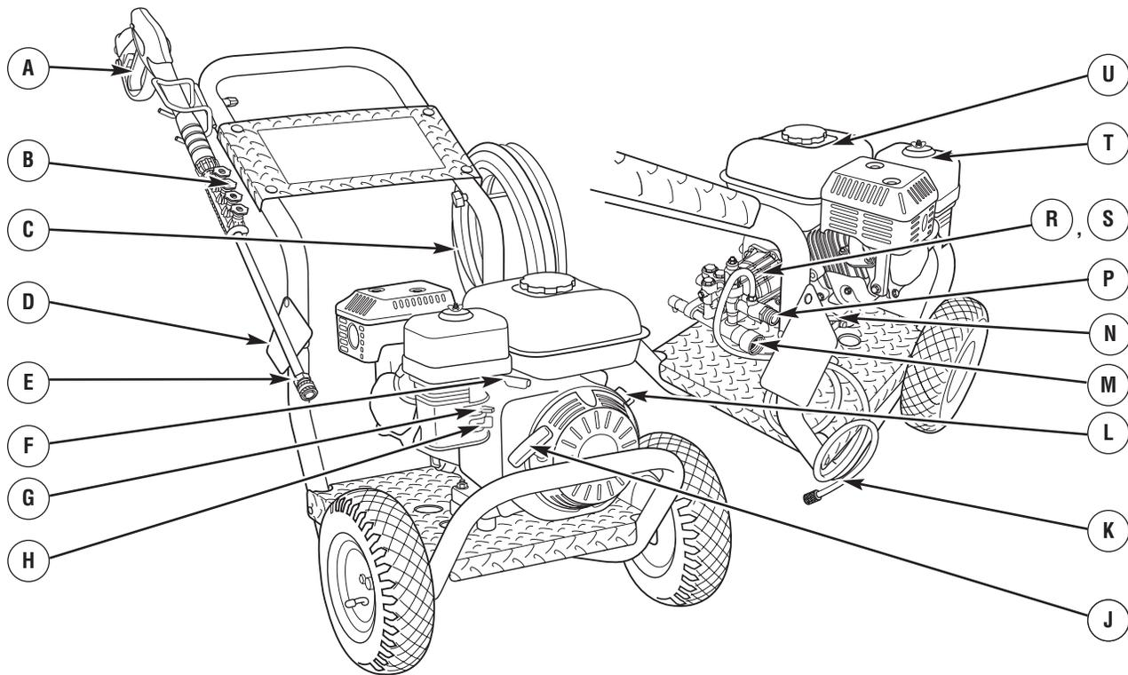
**A - Spray Gun** — Controls the application of water onto cleaning surface with trigger device. Includes trigger lock.
