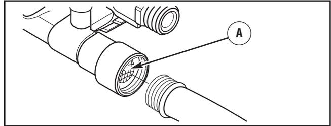
5. Connect the garden hose (not to exceed 50 feet (15 m) in length) to the water inlet. Tighten by hand.
