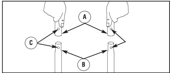
**NOTE:** It may be necessary to move the handle supports from side to side in order to align the handle so it will slide over the handle supports.
