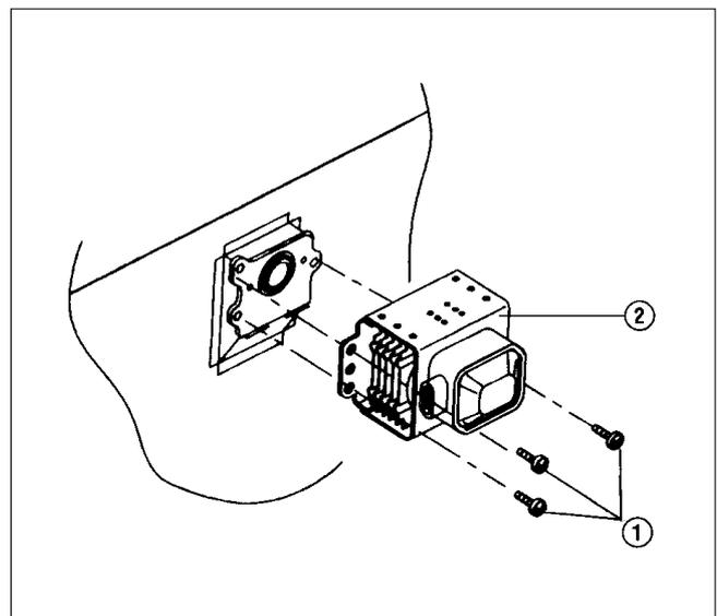
**CAUTION** : Never install the magnetron without the metallic gasket plate which is packed with each magnetron to prevent microwave leakage. Whenever repair work is carried out on magnetron, check the microwave leakage. It shall not exceed  $4\text{mW}/\text{cm}^2$  for a fully assembled oven with door normally closed.
