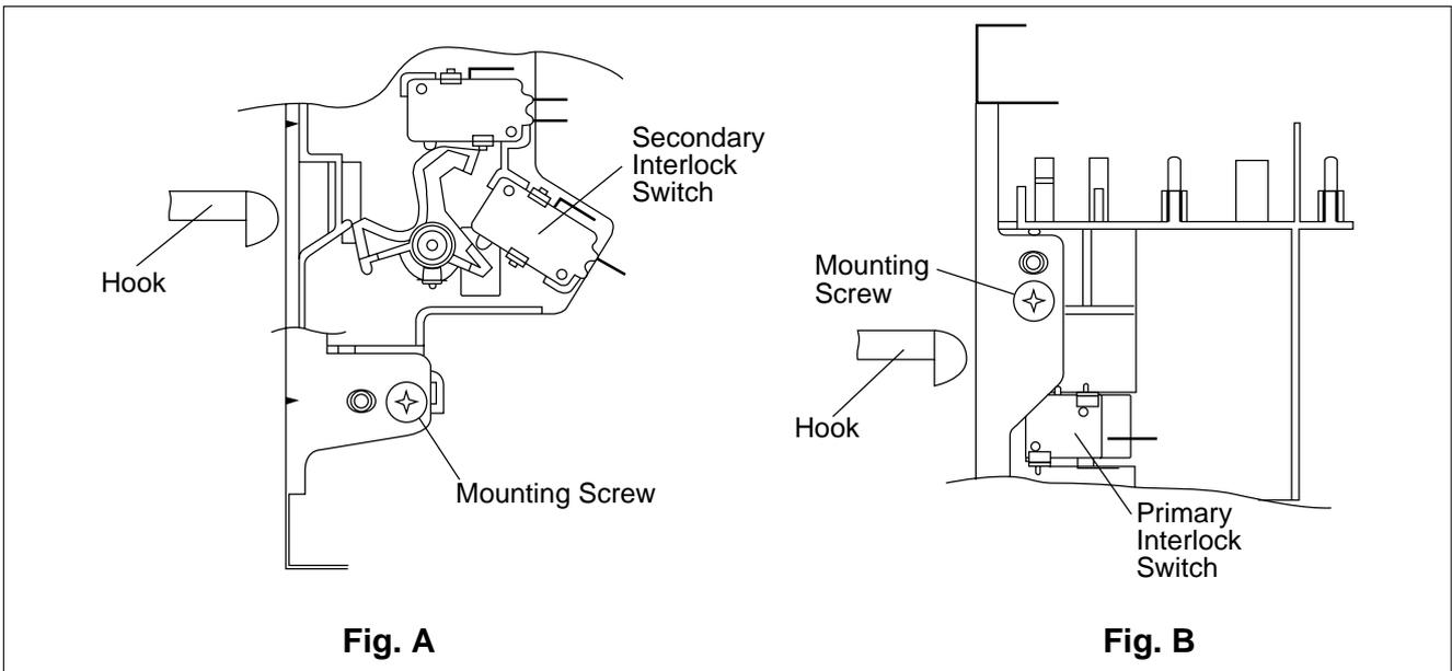
**NOTE :** A small gab may be acceptable if the microwave leakage does not exceed 4mW/cm<sup>2</sup>.
