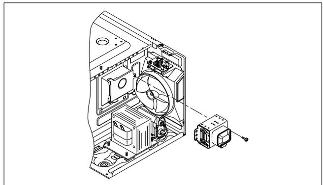
**NOTE :** Never install the magnetron without the metallic gasket plate which is packed with each magnetron to prevent microwave leakage. Whenever repair work is carried out on magnetron, check the microwave leakage. It shall not exceed  $4\text{mW}/\text{cm}^2$  for a fully assembled oven with door normally closed.
