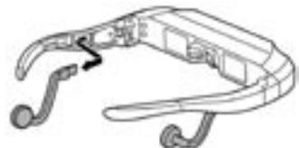
To remove the speakers, pull them out along the inside of the temple piece. Note that the speakers are not designed to fit in your ears.
