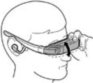
Vuzix' AccuTilt™ technology allows viewer adjustment through 15 degrees to properly align the viewer with your eyes. Grasp the viewer and tilt it until the displays are comfortably aligned with your line of sight. Each temple of the viewer pivots independently for precision adjustment.
