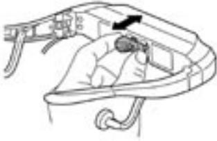
Your iWear® AV920's nose bridge is adjustable for comfort. To adjust the nose bridge grasp it and pull it away from the face of iWear® AV920. The nose bridge can be removed and inserted up-side-down for additional adjustability.
