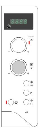
1. Plug the appliance into the mains. The display starts to flash **«00:00»** and then **«REG»**. The dots between the digits blink rapidly.
