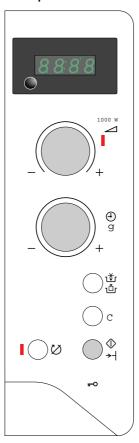
1. Set the required microwave power by turning the power knob. The signal lamp lights up. The time of day disappears from the display and the required microwave power appears: turn to the left = lower power turn to the right= higher power
