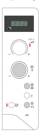
1. Press the button for automatic programmes \*\* \*\* \*\* Until the desired programme appears in the display.
