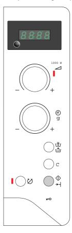
1. Press the START-button three times. The time appears in the display and the programme begins. The microwave power signal lamp lights up.
