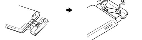
Insert a LR6 (size AA) alkaline dry battery.
