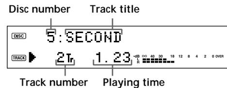
The play mode (e.g., PROGRAM, SHUFFLE) and repeat mode (e.g., REPEAT) shown in the display in Mega CD Control mode indicate the status of the CD changer.
