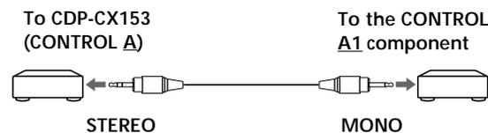
Be sure to connect the STEREO mini-plug to the CONTROL A component and the MONO mini-plug to the CONTROL A1 component.
