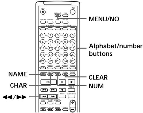
**1** Press NAME repeatedly until a flashing cursor appears in the display, then do the following:
