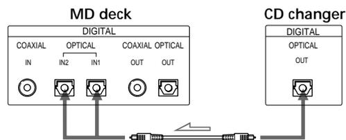
You can connect the optical cable to either OPTICAL IN1 or IN2
