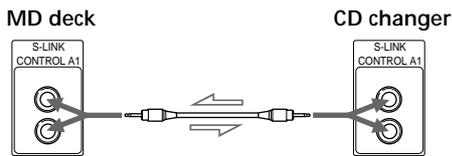
You can connect the cable to either of the jacks
