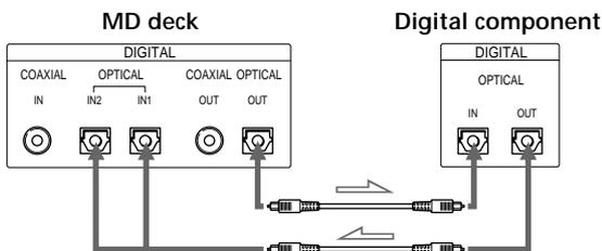
You can connect the optical cable to either OPTICAL IN1 or IN2
