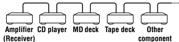
In the CONTROL A1II control system, the control signals flow both ways, so there is no distinction of IN and OUT jacks. If a component has more than one CONTROL A1II jack, you can use either one, or connect different components to each jack.
