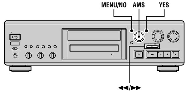
**1** While the deck is stopped, press MENU/NO twice. “Setup Menu” appears in the display.
