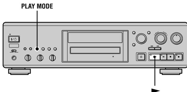
**1** While the deck is stopped, press **PLAY MODE** repeatedly (or **SHUFFLE** once) until “SHUF” lights up in the display.
