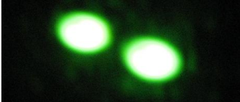
Figure 15 If the beam splits into two when entering the pivot point alignment menu, the pivot point must be adjusted.
