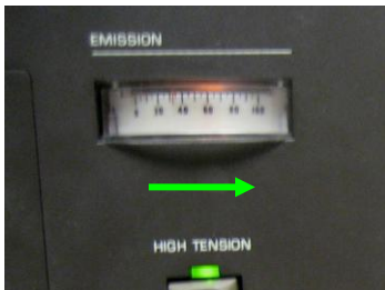
Figure 7 The needle will kick twice to the right after the High Tension button is turned on.
