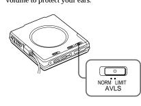
Set AVLS to LIMIT. The volume is kept at a moderate level, even if you try to turn the volume above the
