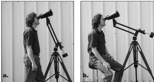
Figure 5. The binocular will remain on target as you adjust the height using the parallelogram. The standing person in (a) is looking at the same thing while seated in (b). Note that only the parallelogram has moved; the tilt angle of the binocular has not. The pivot disk and binocular altitude should not be adjusted for this feature to work.
