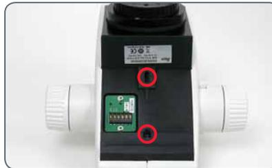
2. Press the optics carrier backwards to the focusing column and screw it in place using your other hand.
