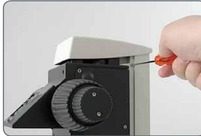
2. Remove the cover of the cable duct.
