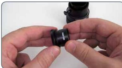
3. Screw the insert and graticule firmly into place and replace the eyepiece in the tube.
