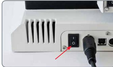
2. Press the on/off switch on the right side once to turn on the illumination.
