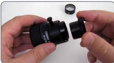
2. Clamp the graticule on the insert, applying moderate pressure. Ensure that the graticule fits tightly.
