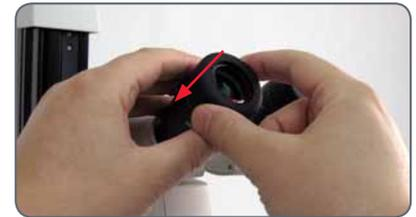
2. If an eyepiece is equipped with the integrated dioptic correction, turn the value to the "0" mark.
