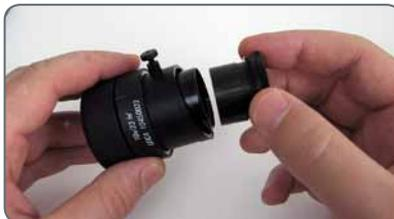
4. You can now align the graticule by rotating the eyepiece in the tube and then tightening it using the clamping screw.
