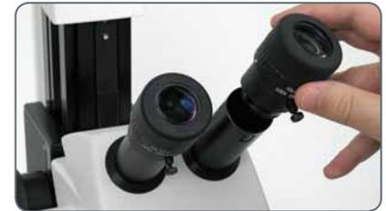
4. Securely tighten the clamping screws.
