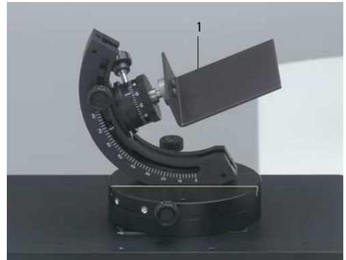
Fig. 45 Adjustable holder with receptacle for locking cylinders
