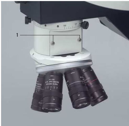
Fig. 9 Fastening the coaxial illuminator 1 Fastening screws for the cover plate
