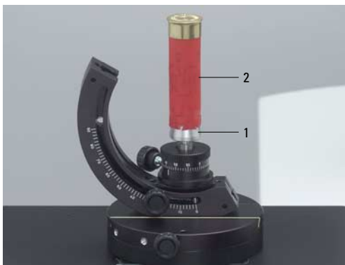
Fig. 43 Adjustable holder with shotgun shell casing holder
