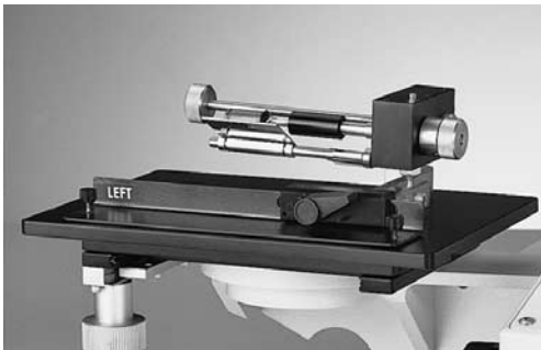
Fig. 50 Cross-stage with attached bullet holder K2715A
