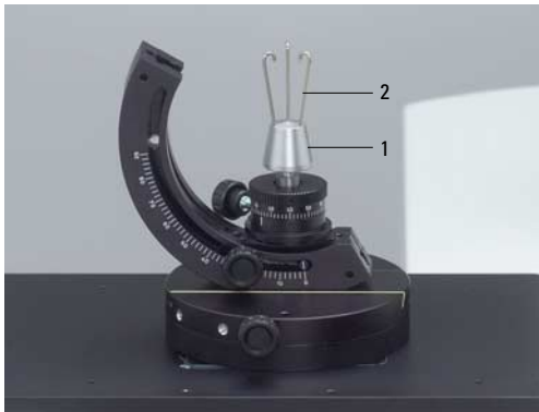
Fig. 43 Adjustable holder with shotgun shell casing holder
