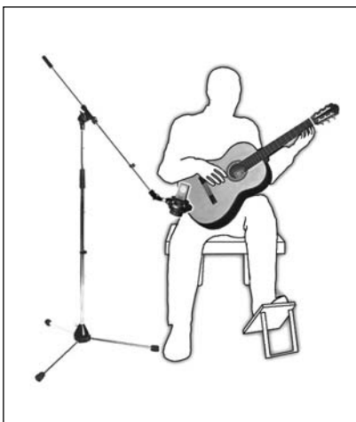
Fig. 8: Miking an acoustic guitar using a single C 414.
