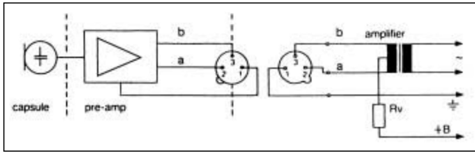
b) circuitry incorporates input transformer **without** centre tap (ungrounded)
