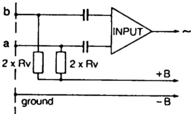
In case where single ended (grounded) amplifier inputs, or where no input transformers are available, either capacitors or optional transformers have to be wired into the audio lines to prevent any current leakage into the input circuitry.
