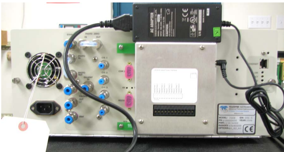
Figure 3-11: T700 Rear Panel Valve Driver Installed
