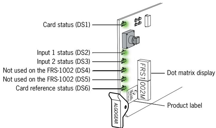
6 status LEDs are located near the FRS-1002 card's front edge. Consult the graphic and color code below to identify the LEDs and their meanings
