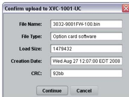
**NOTE:** Pressing the **Cancel** button while uploading will leave the card in an invalid state. Do not click **Cancel** unless the uploading progress has stopped completely for 60 seconds or more. The uploading process can take a few minutes.
