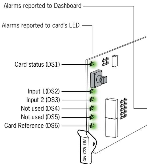
Problems detected by the FRS-1002 card are transmitted as alarms to the card's LED, to the Dashboard interface, and to the optional SNMP monitoring. The problems detected can be reported to the user as minor alarms or critical alarms.
