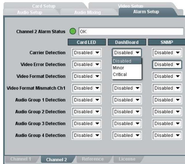
**Minor:** When the alarm level for a specific type or error is set to minor, the card's LED will report the problem with a yellow light and Dashboard with a yellow circle next to an error message describing the problem.
