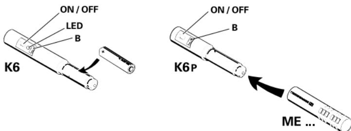
The K6 and K6P powering modules power the various microphone heads of the K6 modular microphone system and provide them with a balanced microphone level output. The powering module is also the microphone body for the different heads. Please refer to the enclosed system overview for possible combinations.
